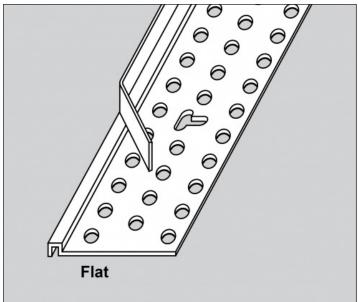
**Description:** Trim-Tex Flat Tear Away is designed to finish edges where drywall terminates at other substrates or building components such as windows and doors.
